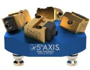
This compact pyramid utilizes four DM25 dovetail fixtures. The small foot print ensures no space is wasted allowing simultaneous machining of four parts. Run more parts per cycle and minimize pallet and tool changes. This versatile fixture can be mounted on trunnions, pallets, and machine tables using our 96mm RockLock Quick Change System.
